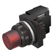
30mm BlackMax, Epoxy Coated Corrosion Resistant Complete Metal Unit Illuminated Indicator Light Transformer type, 480V AC LED Lamp, BA9s Glass Lens, Red UL Listed, CSA Certified NEMA 1,3,3R,4,4X,12,13 & Automotive Standards
