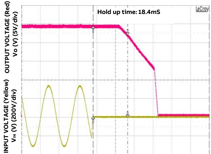
Figure 7. Typical Hold-up Waveforms (VIN = 230V, 100% Load)
