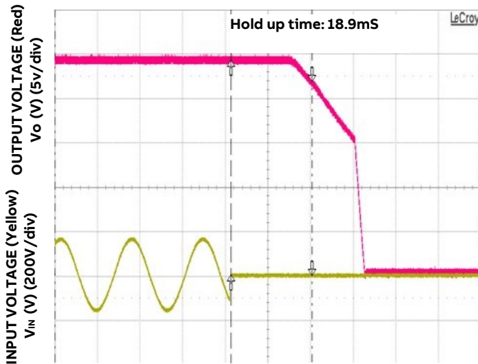
Figure 6. Typical Hold-up Waveforms (VIN = 115Vac, 100% Load)
