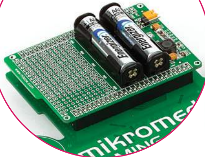
Figure 3-1: Battery Boost shield correctly placed on the gaming shield
