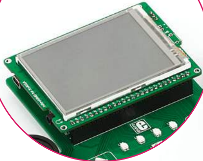
Figure 2-1: mikromedia board correctly placed on the gaming shield
