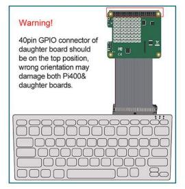
3.Please double check the orientation of daughter board and position of pin#1,2 & 40 base on the below chart before power on Pi400.
