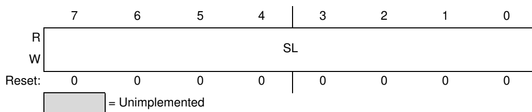
Figure 26. Sensitivity Threshold Register
