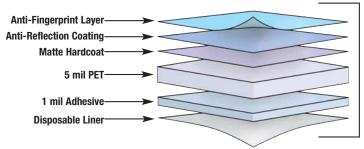
Vikuiti Removable Anti-Reflection Film's unique multilayered construction reduces glare, makes it easier to wipe off fingerprints and helps shield screens from scratches.
