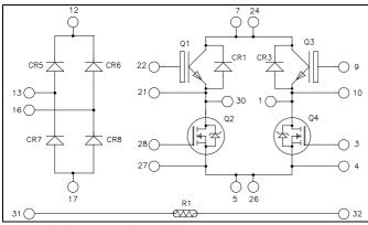
Top switches: Trench + Field Stop IGBT3
