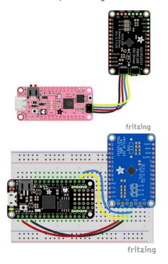
Board 3V to breakout VCC Board GND to breakout GND Board SCL to breakout SCL Board SDA to breakout SDA
