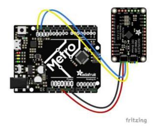
Board 5V to breakout VIN Board GND to breakout GND Board SCL to breakout SCL Board SDA to breakout SDA
