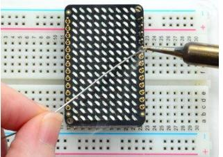
Solder in the two long header strips. Not all are connected on the LED matrix but it makes the connections mechanically stable.
