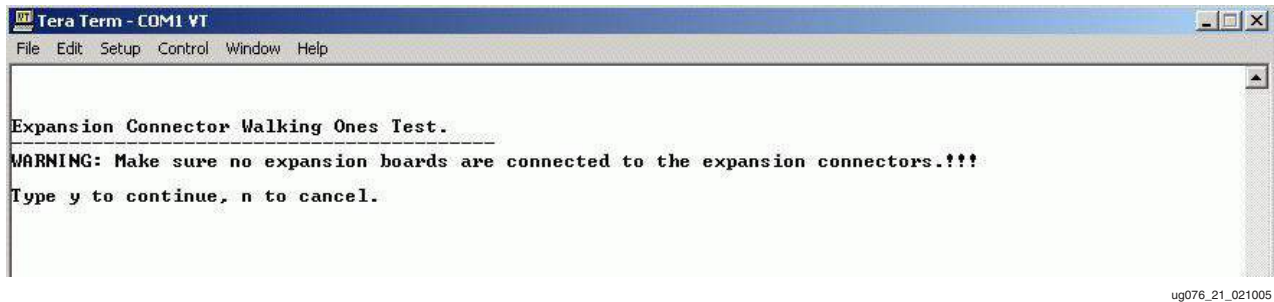
Figure D-21: Confirming Start of the Expansion Port Walking Ones Test
