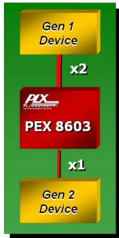
Figure 5. Gen 1 to Gen 2 Bandwidth Bridge
