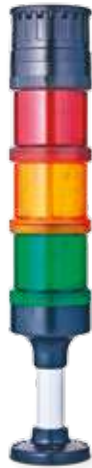
Order number: ECO70-Q81 Colours: red/orange/green Function: LED steady beacon, buzzer steady or pulsing tone Nominal voltage: 230 V AC Type of mounting: Tube mounting (100 mm tube length)
