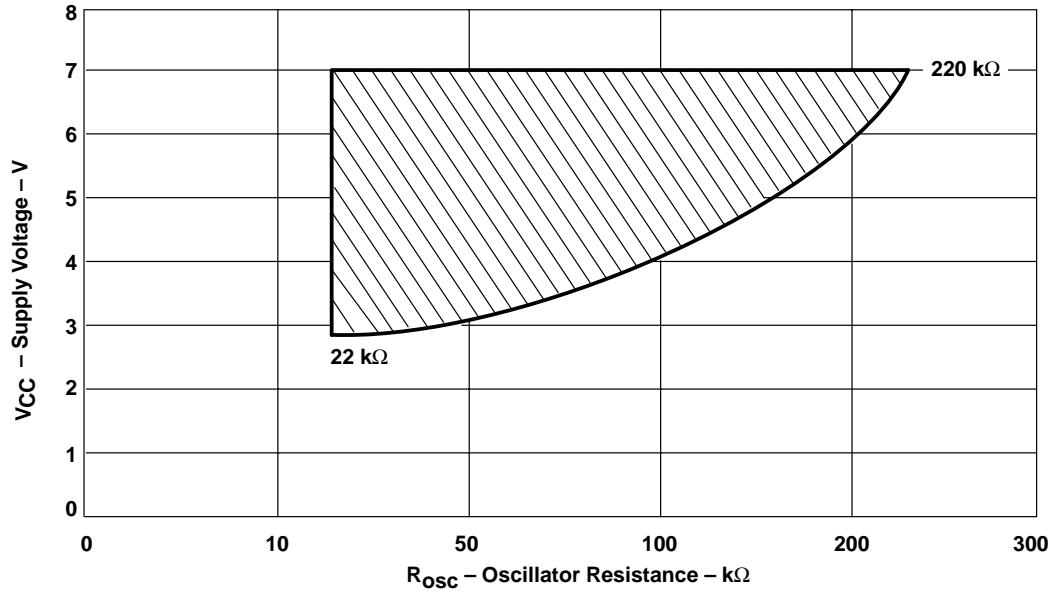
Figure 4-1. Oscillator Resistance Versus Supply Voltage
