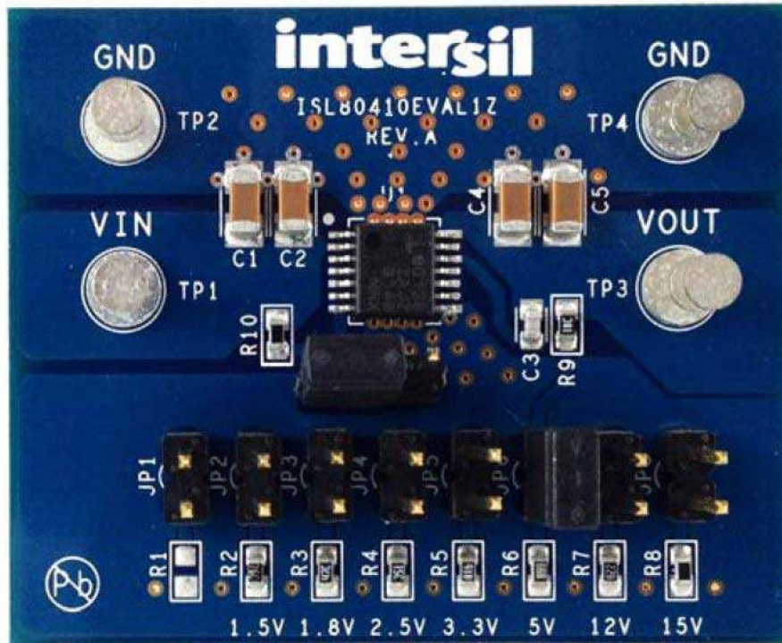
Figure 2. ISL80410EVAL1Z Evaluation Board (Top)
