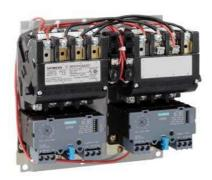
2-speed 3-phase motor starter Size 1 3/4 Two separate windings Constant or variable torque Solid-state overload relays Low SPD OLR range 10-40a High SPD OLR range 10-40a 220-240/440-480VAC 60HZ coil Enclosure NEMA type (open) No enclosure
