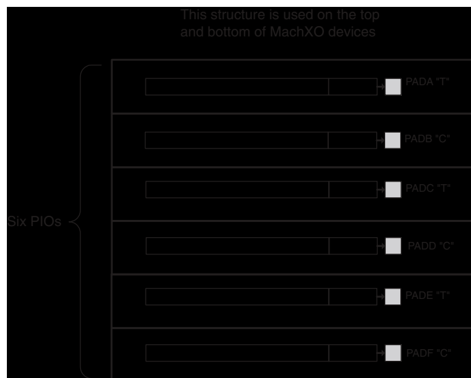
Figure 2-16. Group of Six Programmable I/O Cells
