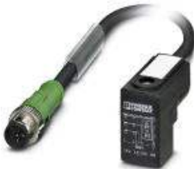
Sensor/Actuator cable, 3-position, PUR, Black RAL 9005, Plug straight M12, A-coded, on C valve plug (8 mm), with 1 LED, connected with Z diode, Cable length: 1.5 m
