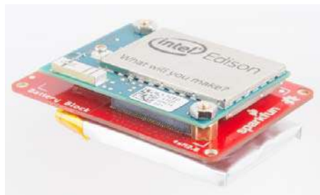
Battery Block Installed
