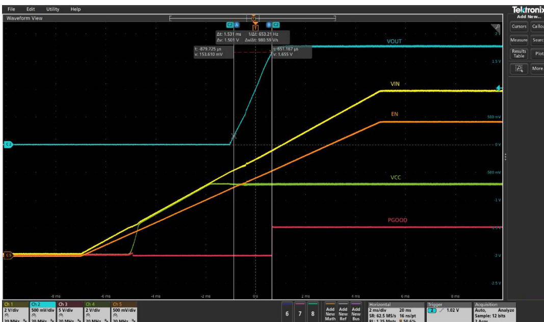
Figure 4 Startup with 6A load (Ch1: PV_{IN} , Ch2: V_{OUT} , Ch3: PG, Ch4: V_{CC} , Ch5: Enable)
