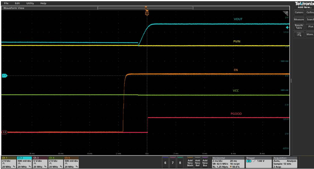
Figure 7 Startup into pre-bias (Ch1:PV IN , Ch2: V OUT , Ch3: PG, Ch4:V CC , Ch5: Enable)
