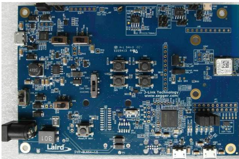
Figure 2: Development board 455-00001 (fitted with 451-00001 BLE module with integrated antenna)
