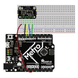
Connect Vin to the power supply, 3V or 5V is fine. Use the same voltage that the microcontroller logic is based off of. Connect GND to common power/data ground Connect the SCL pin to Digital #13 but any pin can be used later Connect the DO pin to Digital #12 but any pin can be used later Connect the SDA pin to Digital #11 but any pin can be used later Connect the CS pin Digital #10 but any pin
