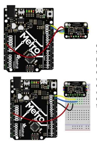
Connect board VIN (red wire) to Arduino 5V if you are running a 5V board Arduino (Uno, etc.). If your board is 3V, connect to that instead. Connect board GND (black wire) to Arduino GND Connect board SCL (yellow wire) to Arduino SCL Connect board SDA (blue wire) to Arduino SDA
