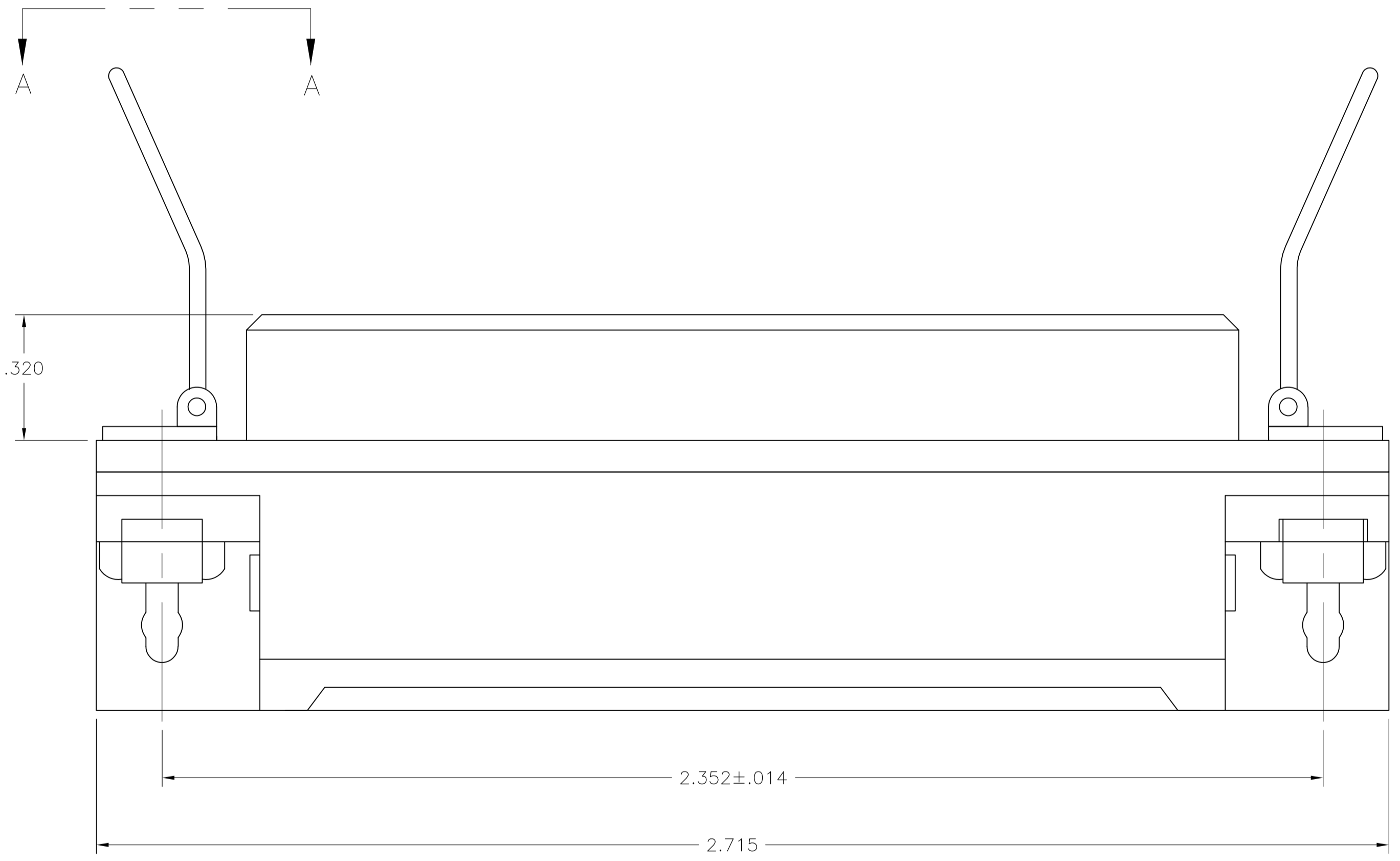
SUGGESTED PRINTED CIRCUIT BOARD MOUNTING DIMENSIONS
