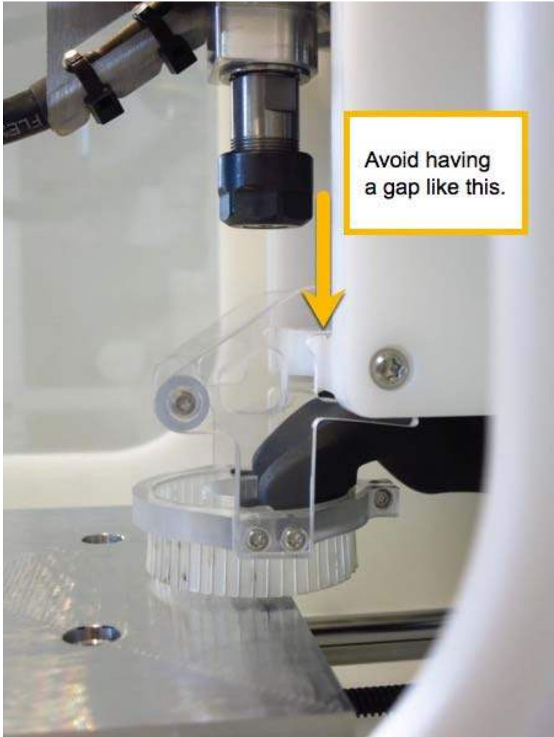
Incorrectly installed Dust Collector Hood: Avoid having a gap between Dust Collection Hood arms and X Carriage frame
