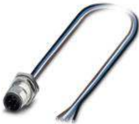
Panel feed-through, 4-position, Flush-type plug, straightLink:M12-SPEEDCON, A-coded, Rear mounting, M12 x 1, Individual wires, Cable length: 0.5 m
