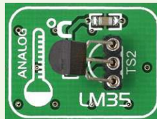
Figure 21-2: LM35 correctly placed in socket
