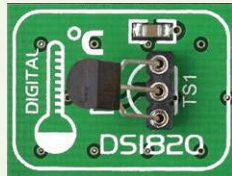
Figure 20-2: DS1820 correctly placed in socket
