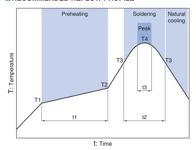
Preheating Soldering Peak Time Temp. Temp. Time Temp. Time T1 T2 Т3 **T4** t3 150°C 180°C 90 to 120s 230°C 40s 255°C 10s max.
