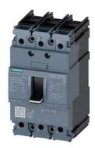
circuit breaker 3VA5 UL frame 125 breaking capacity class H 65kA @ 480 V 3-pole, line protection TM210, FTFM, In=90A overload protection Ir=90A fixed short-circuit protection li=10 x In nut keeper kit on both sides
