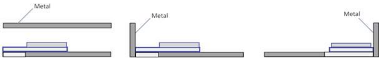
Figure 5-4. Not recommended location in Z plane
