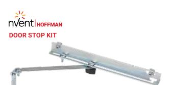
Door Stop Kit secures the door in the open position. Kit can be installed at the top or bottom of a door which opens horizontally. Door opening angle can be easily adjusted by means of a wing nut. Stop arm slides neatly out of the way when the door is closed. All parts are plated. Mounting hardware included.
