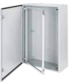
Swing-Out Rack Frames provide 120-degree swing-out access for 19-in. rack equipment. Welded rack frame mounts to front flange. Distance from frame to door surface is 1.32 in. (33 mm) for solid doors and 1.07 in. (27 mm) for window doors. Frame is painted white. Mounting hinge and latching hardware provided. Order separately clip nut package catalog number XNM5 and screws XSM5 (metric) or AN1032 and screws AS1032 (English). Swing-Out Rack Frame cannot be mounted on adjustable mounting kit.
