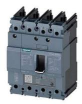
circuit breaker 3VA5 UL frame 125 breaking capacity class S 25kA @ 480V 4-pole, line protection TM230, FTAM, In=90A overload protection Ir=90A fixed short-circuit protection Ii=5...10 x In N conductor protection 100% without connection
