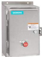
Non-reversing motor starter Size 0 Three phase full voltage Solid-state overload relay OLRelay amp range 3-12A 550/575-600 50/60HZ coil Combination type Water/dust tight non-corrosive
