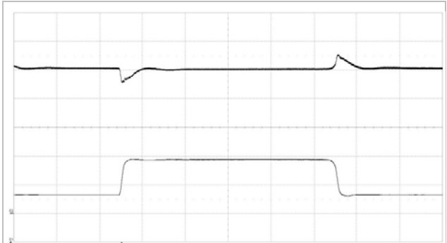
Output voltage response to load current step-change (12.5-37.5-12.5 A) at: T_{P1} = +25^\circ\text{C} , V_I = 53\text{ V} , C_{out} = 2.2\text{ mF}
