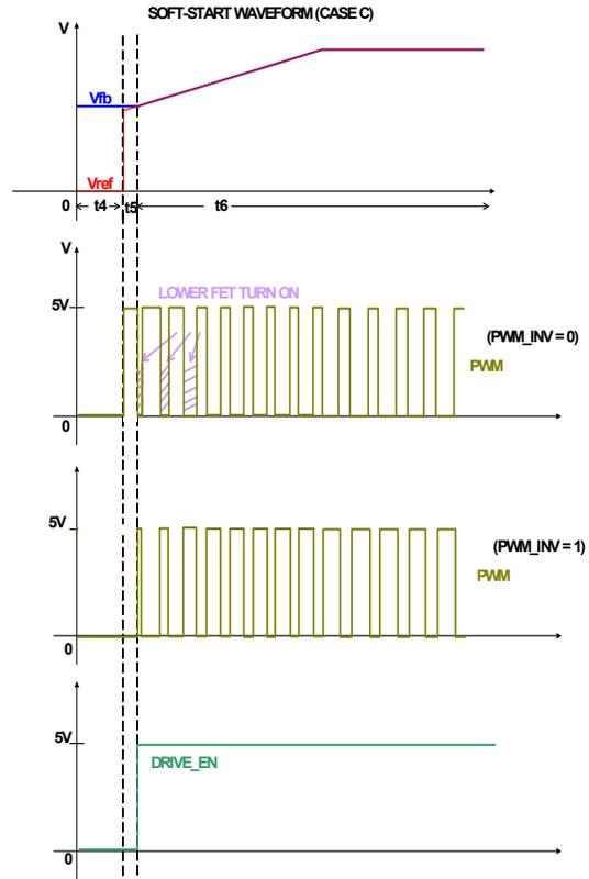
FIGURE 17. SOFT-START WAVEFORM (CASE C, LIGHT LOAD)
