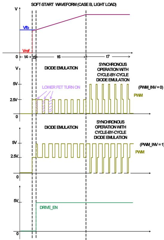
FIGURE 16. SOFT-START WAVEFORM (CASE B, LIGHT LOAD)
