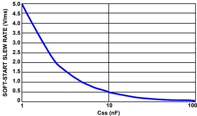
FIGURE 18. SOFT- START CAPACITOR vs SLEW RATE
