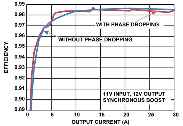
FIGURE 3. 11V INPUT EFFICIENCY vs OUTPUT CURRENT vs PHASE DROPPING MODE
