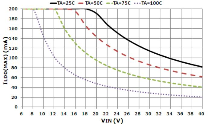
FIGURE 22. I<sub>LDO(MAX)</sub> vs V<sub>IN</sub>
