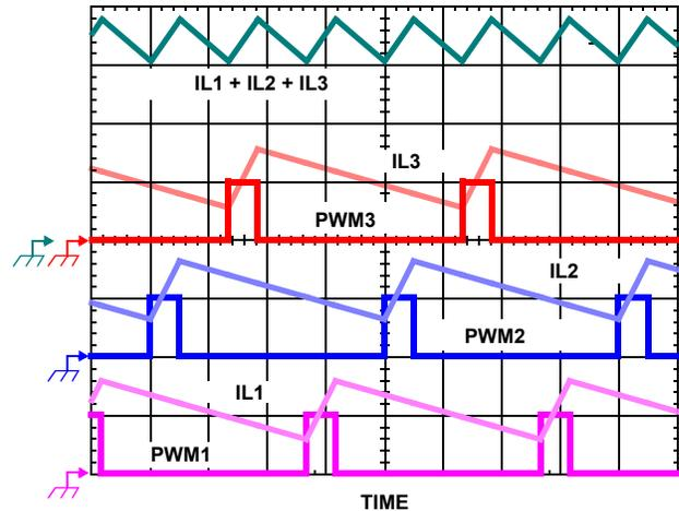
FIGURE 13. PWM AND INDUCTOR-CURRENT WAVEFORMS FOR 3-PHASE CONVERTER
