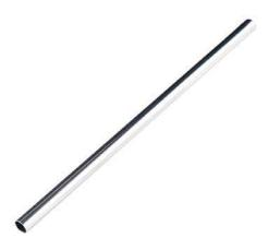
**Description:** These 12" long aluminum tubes have an outer diameter of  $\frac{1}{2}$ ", an inner diameter of 0.444", and a wall thickness of 0.03". When used with the mating tube clamps, these can be used for versatile structural support. Additionally, wires and cables can easily be run through the center.
