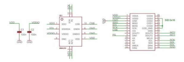
BMA280 shuttle board electrical layout
