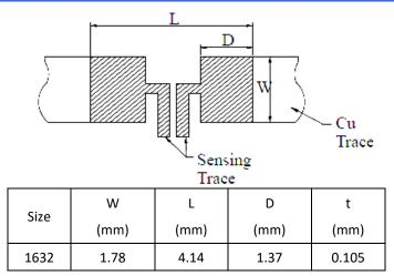
t: Copper toil minimum thickness of PCB
