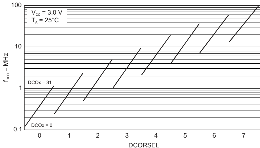
Figure 8-10. Typical DCO Frequency
