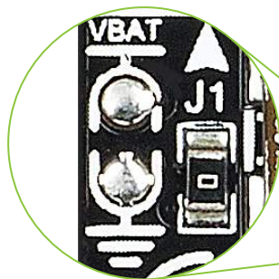
Figure 6-1: battery pads and jumper J1
