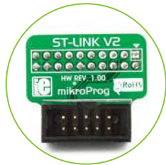
Figure 4-11: mikroProg™ to ST-LINK™ V2 adapter
