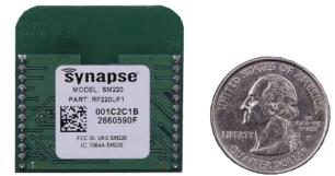
Each **SNAP Engine** combines a microcontroller, a radio, and an antenna. The antenna can be an integral "F" antenna, or a mounting point for an external antenna. The **SNAP Engines** included in your **EK2100-220** evaluation kit are **RF220-UF1 SNAP Engines**, (also known as **RF220 SNAP Engines**), as pictured above. **RF220 SNAP Engines** communicate using 802.15.4, 2.4 GHz radio signals.
