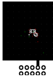
c) 86^\circ\text{C/W} when mounted on a 1\text{ in}^2 pad of 2 oz copper
