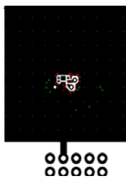
a) 86^\circ\text{C/W} when mounted on a 1\text{ in}^2 pad of 2 oz copper
