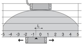
5 mm misalignment tolerance after setting
