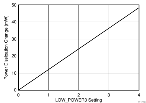
Figure 8-13. Power Dissipation Change vs LOW_POWER3 register setting
