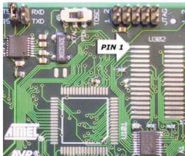
Figure 2-9. Pin1 on SRAM Footprint and Pinout
