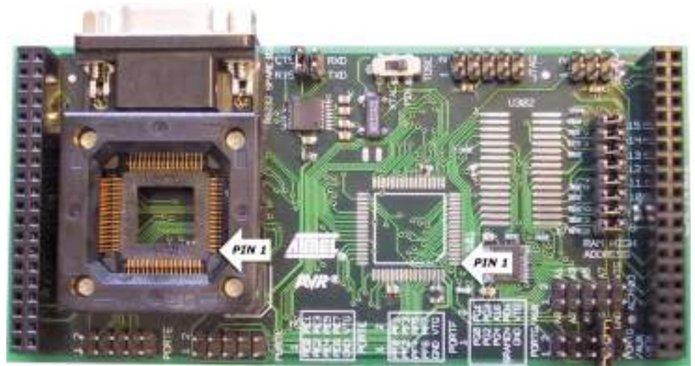
Figure 2-2. Pin1 on ZIF Socket and TQFP Footprint
