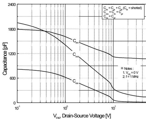
Figure 5. Capacitance Characteristics
