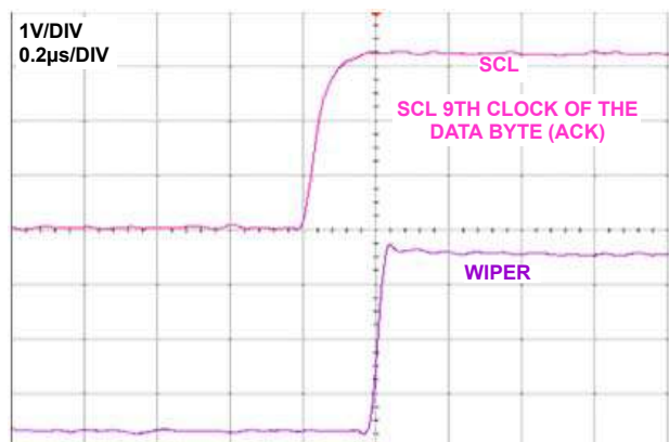
FIGURE 21. WIPER LARGE SIGNAL SETTLING TIME
