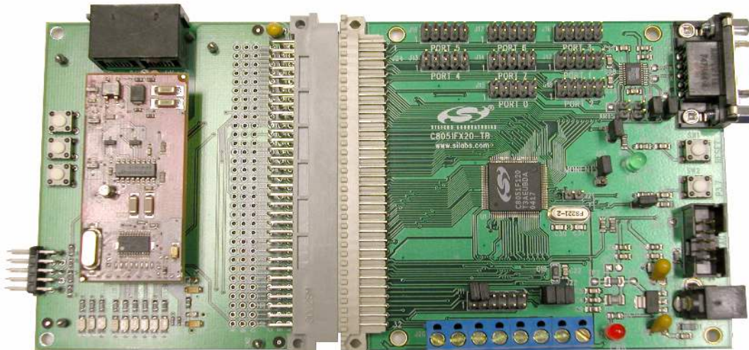
Figure 1. Embedded Modem Development Kit Hardware Overview
