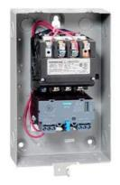
Non-reversing motor starter Size 1 3/4 Three phase full voltage Solid-state overload relay OLRelay amp range 10-40a 190-220/220-240V 50/60HZ coil Combination type Indoor general purpose use
