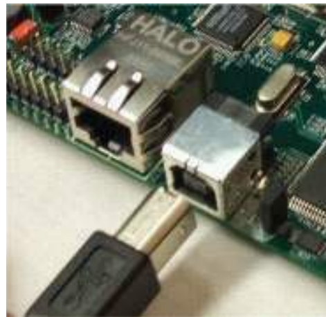
Figure 4-4: Connect the USB Type B Connector to the MicroBlaze Development Kit Board Connector
