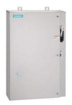
Non-reversing motor starter Size 4 Three phase full voltage Solid-state overload relay OLRelay amp range 50-200A 110V 50HZ / 120V 60HZ coil Combination type 200A fusible disconnect 200A/600V fuse clip Encl NEMA type 4X 316 S-steel Water/dust tight noncorrosive Standard width enclosure
