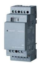
SIPLUS LOGO! AM2 RTD based on 6ED1055-1MD00-0BA2 with conformal coating, -40...+70 °C, start up -25 °C, extension module, PS: 12/24 V DC, 2 AI - 50...+200 °C Pt100/1000 for LOGO! 8
