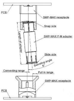
The connecting range represents the maximum misalignment during connection.
